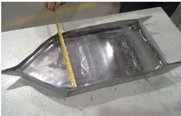
Fig. 2. Manually produced crucible with the sapphire ingot after the crystallization process.
