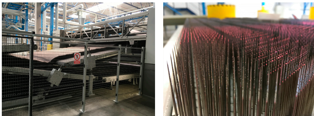
Figure 2. Semi-finished product layered in several layers (left) and detailed view of the needles (right).
