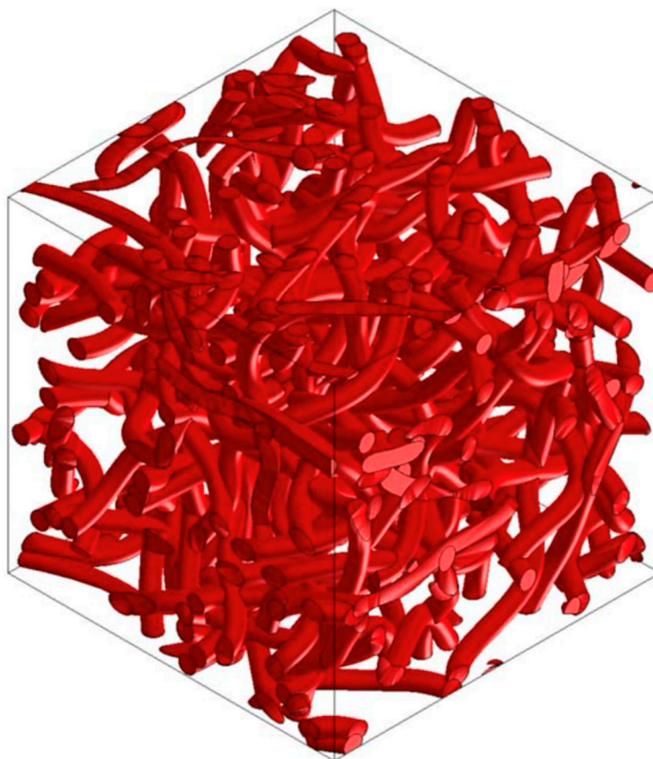
Figure 22. RVE geometry for a composite made from PP/PET/cotton—60/0/40.
