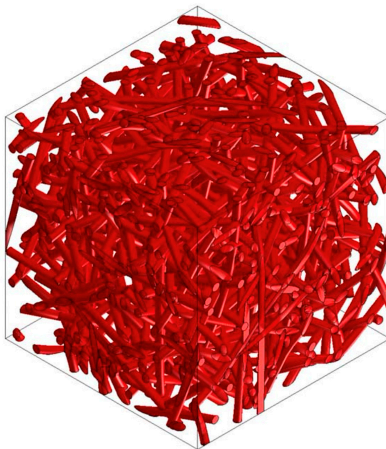
Figure 24. RVE geometry for a composite made from PP/PET/glass fibers—60/0/40.
