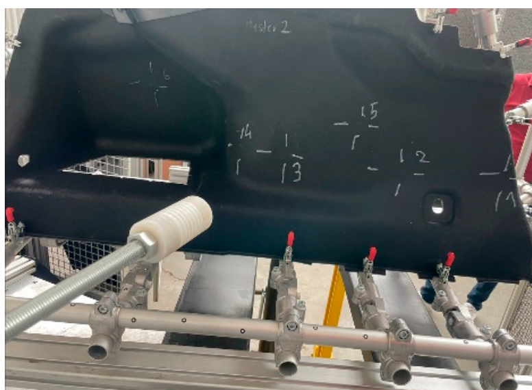
Figure 8. Example of the location of the measuring attachment for various testing points from MP1 to MP6.
