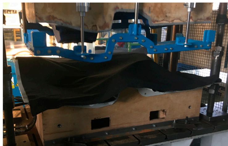
Figure 3. View of the production of composite material for the luggage compartment of a car.
