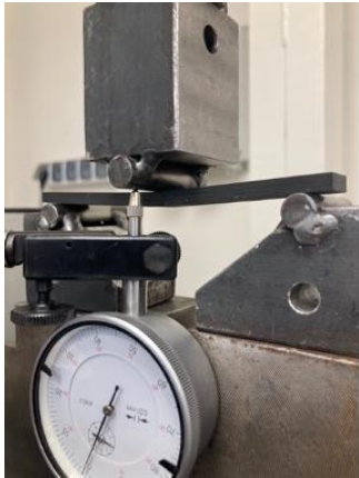
Fig.7, The 3-point bending test, composite sample with dimensions 100x10x5 mm using the test equipment LABTEST 1052
